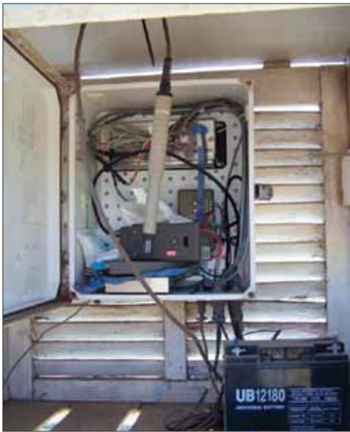
Figure 4. Temperature station at the Chico University Experiment Farm. Who puts a temperature sensor right next to heat-generating electronics?
