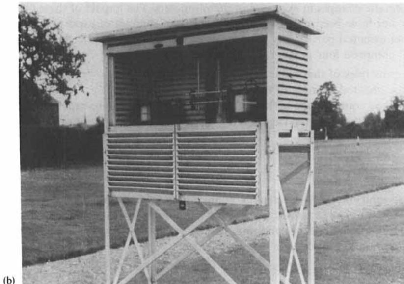
Figure 1. (a) Stevenson screen, old version (from Mawley, 1897) © Royal Meteorological Society. (b) Modern Stevenson screen © HMSO
